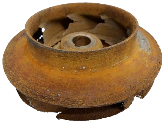
A METALLIC IMPELLER AFTER ONLY 3 MONTHS OF OPERATION IN FRESH WATER!
