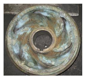
Original Bronze Impeller showing damage from Corrosion, Erosion, and Cavitation
