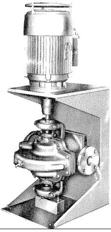
Figure 3. The old design of the Metallic Double-Suction Pump
