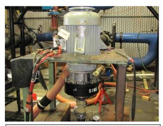
The SIMS MCM Fire Pump on a test rig in California prior to installation on board the mine sweeper.
