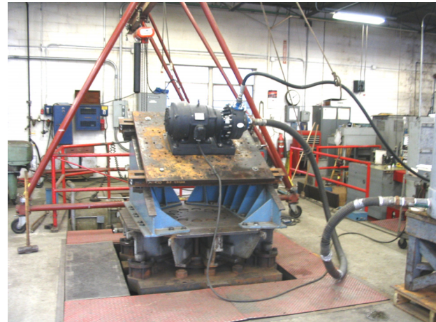
Pump Shaft Perpendicular to Incline Axis
