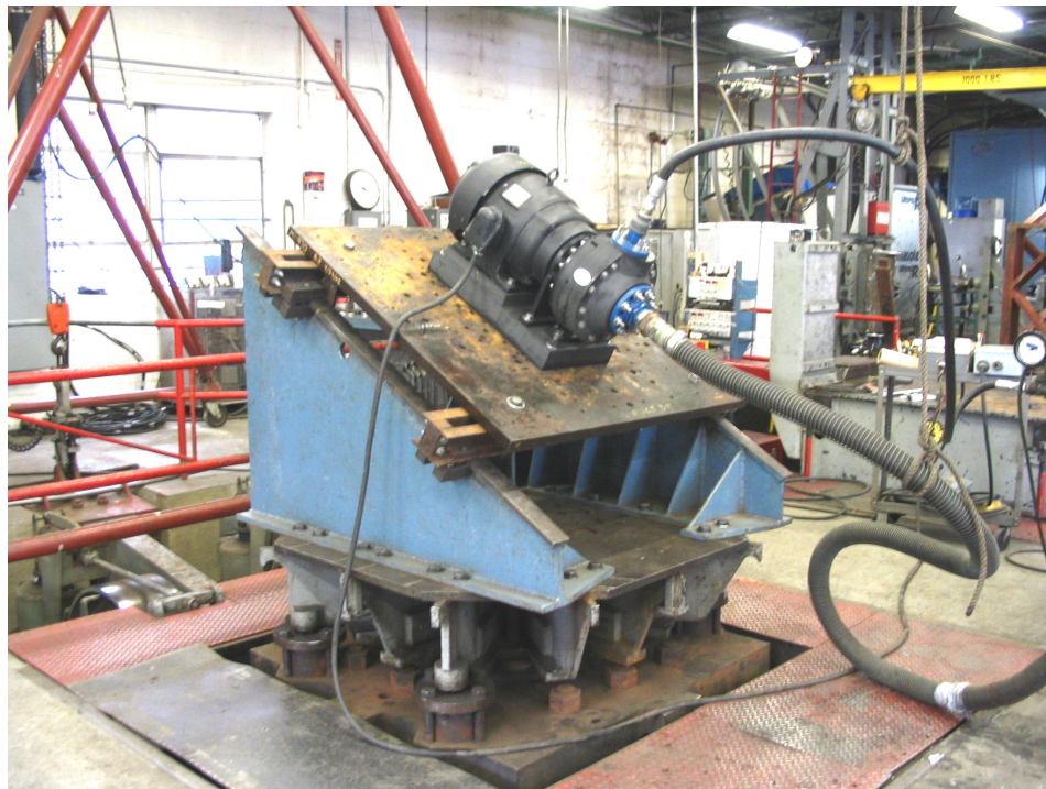
Pump Shaft Parallel to Incline
