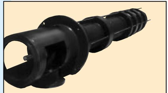
The above vertical turbine screen wash pump is manufactured with Permalube® Spider Bearings, Throttle Bushing and Guide Bearings. One of the biggest advantages of the Permalube Bearing is its ability to take dry start up until the fluid reaches the bearing to lubricate the surfaces. Permalube® Bearings have graphite and PTFE built into the resin system
