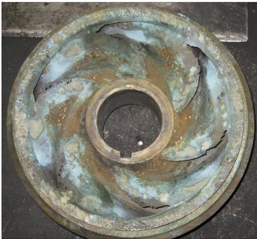
**Original Bronze Impeller showing damage from Corrosion, Erosion, and Cavitation**
