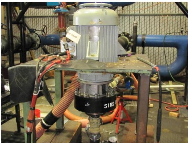
The SIMS MCM Fire Pump on a test rig in California prior to installation on board the mine sweeper.
