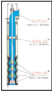
to enable these bearings to endure dry running on start-up. This pump was manufactured by the Sims Pump Company for a major power utility company in Maryland.
