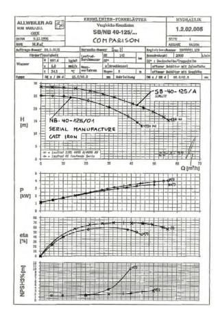
Below is a chart compiled by Kumho-Mitsui, which looked at the ROI of a standard production metallic impeller compared to a Structural Graphite Composite Simsite® Impeller obtained from SIMS Pump Company, an aftermarket centrifugal pump manufacturer. It is clear from the test report that the upgraded aftermarket impeller reduced energy consumption by 10%.
