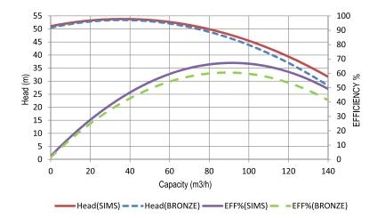
The above graph shows that changing the Bronze Impeller to a Simsite® Structural Composite Impeller increased efficiency 15.8%! The efficiency on this 20 KW pump (26.8 HP) went from 57% with a metallic impeller to 66% with a structural composite impeller — an increase of 9 points or 15.8%! At 0.11 cents per kilowatt hour this translates into a yearly savings of \$2,218.00 per year, per pump!
