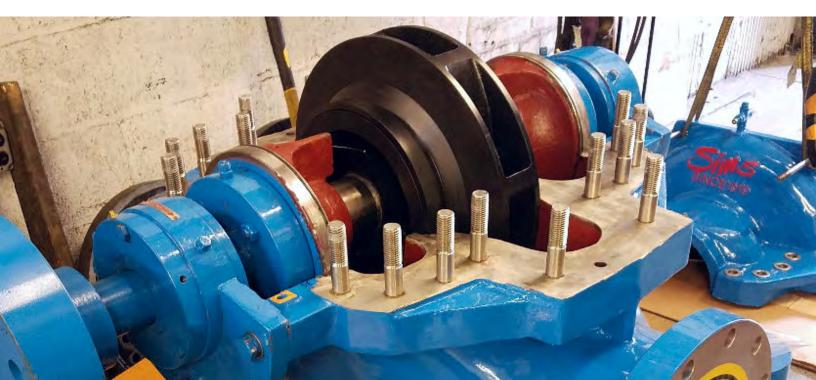
SIMS PUMP also installed two (2) of their patented SIMSITE® Structural Composite Stabilizing Bushings on each side of the impeller in the seal chambers next to the mechanical seals to further increase the longevity of the seals and bearings by reducing shaft deflection and axial movement!
