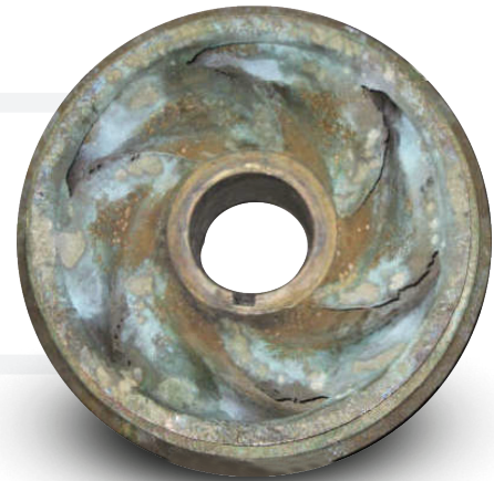
Original Bronze Impeller for the central salt water cooling pump, size 16," showing damage from Corrosion, Erosion, and Cavitation.
